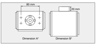
\* For rotary process valve actuator with standard attachment to VDI/VDE 3845 with A = 80 mm, B = 20 mm
